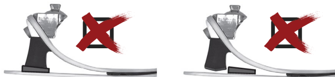
Improper Wedge Placement
